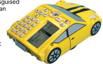
**Pro-Bot** is self-contained, controlled via the on board keyboard, with no need for an additional device or managing a connection. The built-in LCD screen displays the code as commands are entered. Press GO and watch Pro-Bot follow each command as it is highlighted on the screen. Need to make a change? Use the edit keys to make an adjustment right on the screen.
