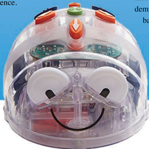
Transparent shell to show inner workings
